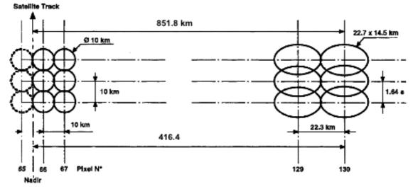
Figure 1: pixel representation on the ground for SAPHIR.
