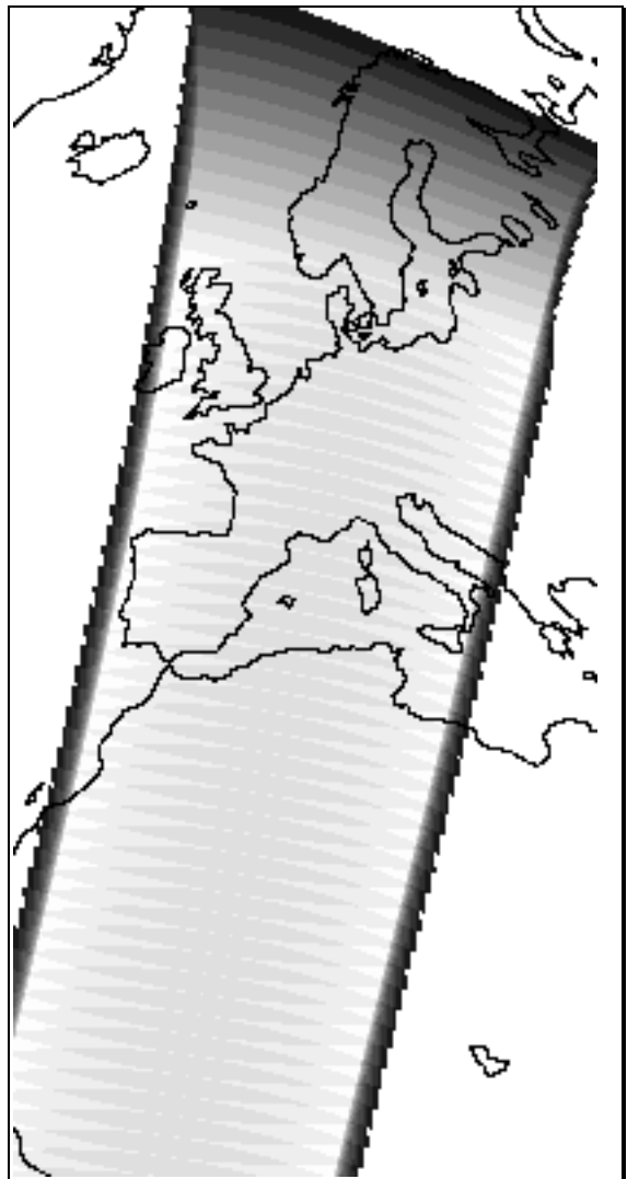
Fig. 3 : Number of viewing directions available for each surface pixel. Gray shades are from one (Black) to sixteen (white). Fourteen directions are available in the wide area around the satellite subtrack
