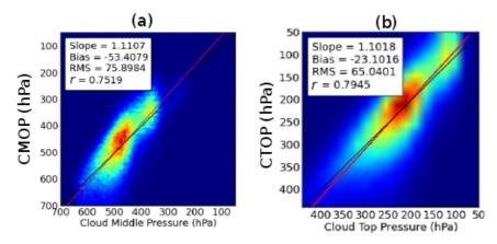
Figure 1: Evaluation of POLDER cloud middle and top oxygen pressure (CMOP on panel (a) and CTOP on panel (b)) against CPR/CALIOP cloud middle pressure (in abscissa). Cloud cases over ocean in 2008. Black lines indicate the one-to-one relationship, while red lines indicate the linear regression between CMOP and CMP.
